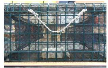
**Photograph of the basic style of trap used for sampling of juvenile fish on a cobble and boulder reef in L.I. Sound.**
