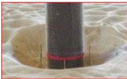
**Local scour: The erosion of seabed material in proximity to a single foundation, e.g. a monopile or a single leg of a jacket foundation (From Epsilon, 2018)**
