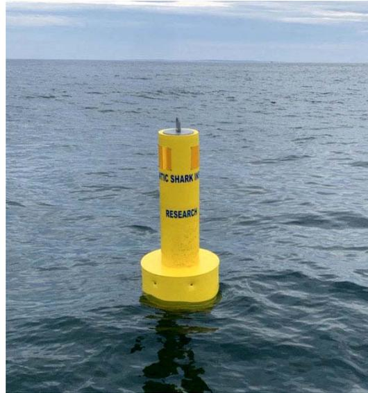
Our suspicion is that the anchoring chain may have disconnected from the mushroom anchor so it is highly likely that the receiver is still attached to 115 feet of chain. As a result, it may have gotten hung up anywhere in the region.
